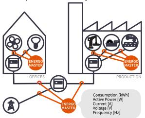
Data measured by Energomaster is sent via a communication interface (WiFi, 2G, NB-IoT, *LoRaWAN*, etc.) to monitoring and management systems at adjustable intervals (5 seconds – 60 minutes).
